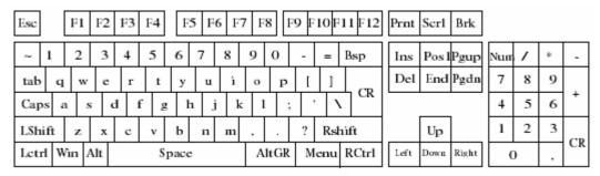
Figure B.1: English (US) Keyboard Layout, used for key codes
